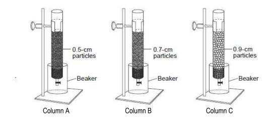
Water was poured into each tube and the time the water took to travel between the dashed line and the bottom of the tube was recorded. Each column was tested 3 times.
