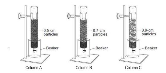
Water was poured into each tube and the time the water took to travel between the dashed line and the bottom of the tube was recorded. Each column was tested 3 times.
