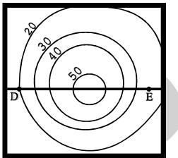
Construct a grid with a baseline the same distance as the profile you wish to draw. Label the baseline with the correct letters (in this case "D" and "E".)
