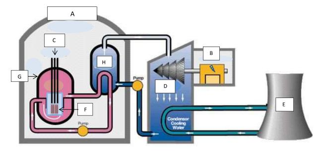
3. How does forced nuclear fission work? Label the key components of the fission diagram shown below.
